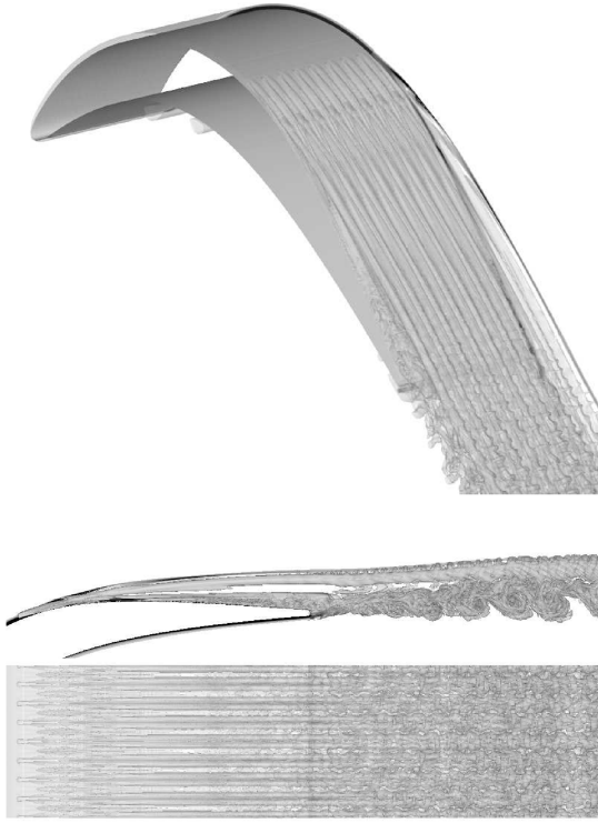
Fig. 33 Fine grid solution. Streamwise vortices with spanwise wavelength, \lambda_z = 0.05 , and amplitude A = 10 . Isosurfaces of vortex identification criterion, Q = 1 , and isocontours of spanwise vorticity, \omega_z , at z = 0 . From top to bottom: perspective view of blade, side view of wake, and top down view of wake. Computational domain was repeated once in spanwise direction.
