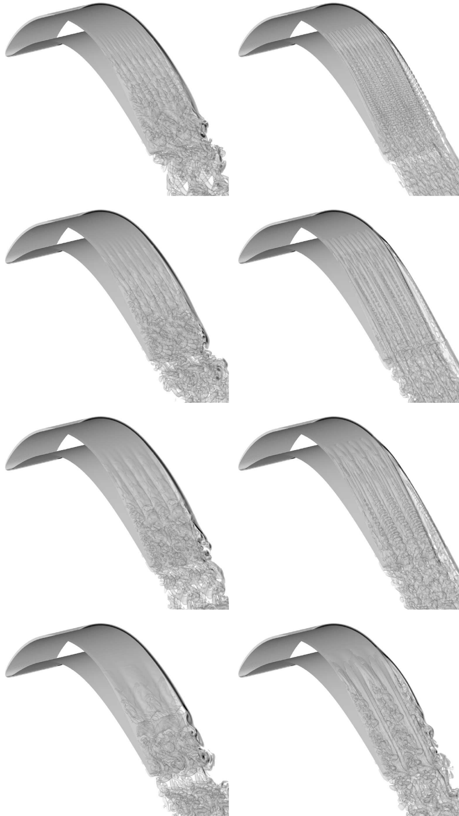
Fig. 28 Streamwise vortices with spanwise wavelength, \lambda_z = 0.05, 0.0667, 0.1, 0.2 (top to bottom), and amplitude A = 1 (left) and A = 10 (right). Isosurfaces of vortex identification criterion, Q = 1 , and isocontours of spanwise vorticity, \omega_z , at z = 0 . Computational domain was repeated once in spanwise direction.
